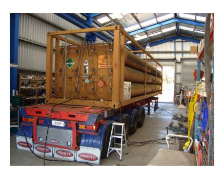
n the compressed gas tube industry, it is the general standard that government regulators require that all tubes are retested and/or recertified every 5 years using a hydrostatic test and volumetric expansion test. These testing methods have been the standard globally to ensure that equipment required for gas transport and storage are in tip-top condition. TISEC Inc.
