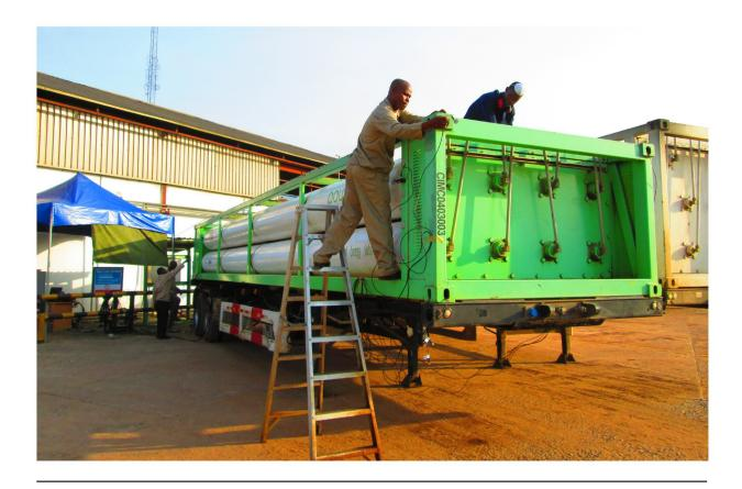
Tektrend International Inc. The company took on a joint research project to develop an acoustic emission test procedure for recertification of tube mounted trailers that were used to transport compressed gas. Tektrend collaborated with Air Liquide Canada and Air Liquide France, Transport Canada and US DOT for this project.
